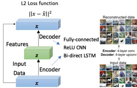
Figure 3. VAE training process such that the features can be used to reconstruct the original data
