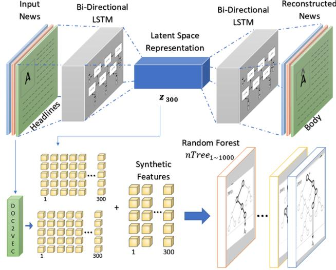
Figure 2. The overall architecture of the proposed high dimensional latent space framework
