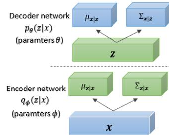
Figure 4. The probabilistic components: Mean and diagonal covariance of  $\mathbf{z}|\mathbf{x}$  and  $\mathbf{x}|\mathbf{z}$  of the Gaussian encoder and decoder
