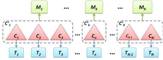
Figure 3. Architecture of the two-layer classifiers. The dashed rectangles indicate the middle classes which consist of different numbers of target classes
