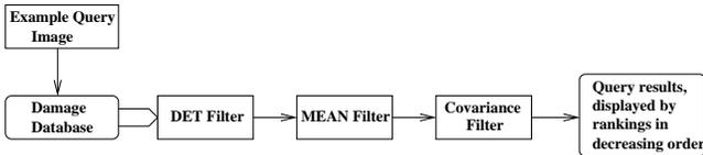
Figure 5: The multi-filter query architecture.
